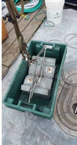
Figure 11: WILDCO Ponar Grab Sampler
