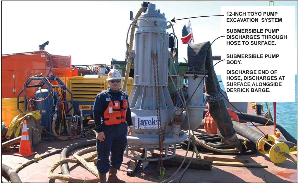
TOYO PUMP EXCAVATION SYSTEM SHOWN RESTING ON DECK OF BARGE READY FOR DEPLOYMENT. THE PUMP IS ELECTRICALLY POWERED BY A GENERATOR OPERATING ON THE DECK OF THE BARGE. A DIESEL POWERED JET PUMP IS USED TO PROVIDE JET WATER THAT IS USED BY THE SYSTEM'S WATERJET SYSTEM.
