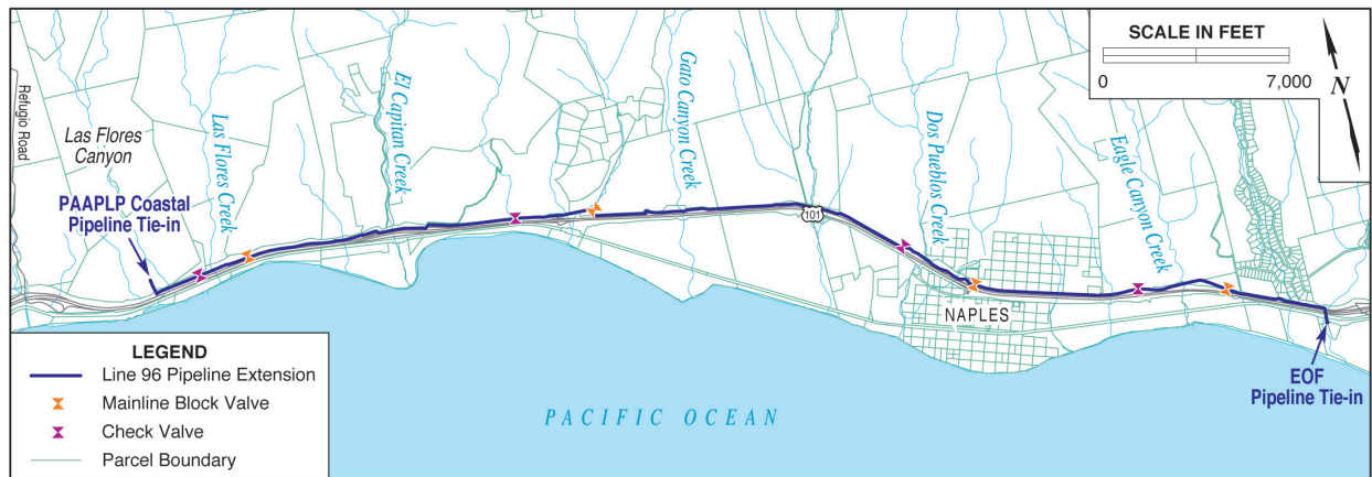
Figure 2-7. Line 96 Pipeline Route
