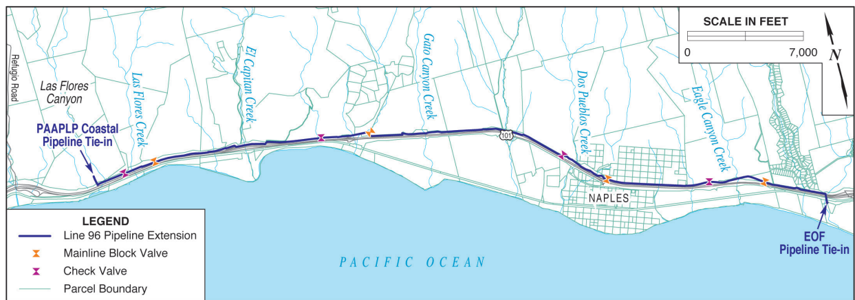
FIGURE ES-2. LINE 96 PIPELINE ROUTE
