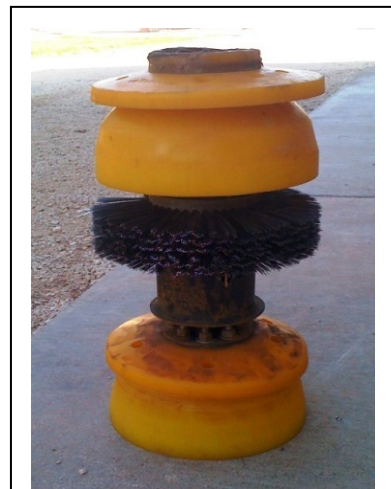
Illustration 2-2. This photo shows a cleaning pig for a 6-inch oil pipeline. The wire brush encircles the shaft and scours the interior of the pipeline. (Photo: Berg 2009.)
