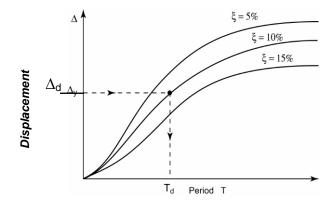
Figure 31F-4-4--Design Displacement Response Spectra
