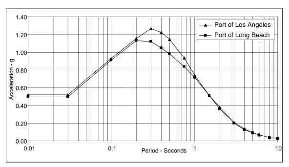
FIGURE 31F-3-1 - DESIGN ACCELERATION RESPONSE SPECTRA FOR
